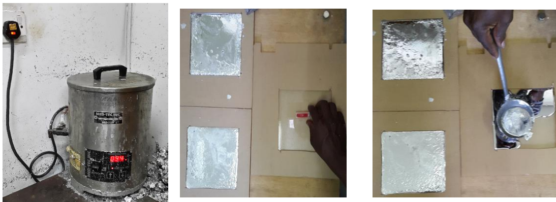
Plate 3.01. Alloy melter used in this work to melt cerrobend
