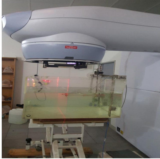
Plate 3.08. Experimental setup used for determination of factors to account for reduction in scatter for using bolus on the surface to be mimicked by cerrobend on block tray.
