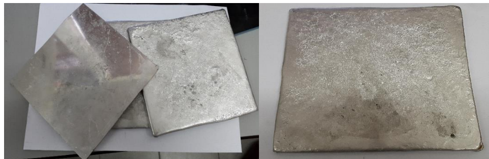
Plate. 2.01. Cerrobend slabs produced in this present research and used in the measurements for determination of linear attenuation coefficient
