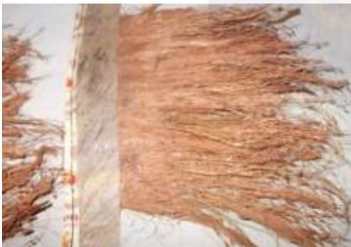
Fig. 24 A sleeve prepared from the coir.
