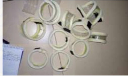
Fig. 48 Plastic bottles converted into Shackles.
