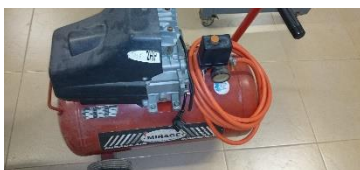
Figure A 7 Air compressor
