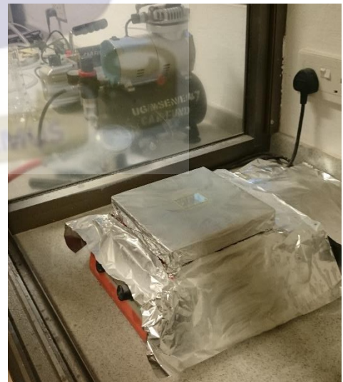
Figure A 3 Glass slide on hot-plate during spray deposition
