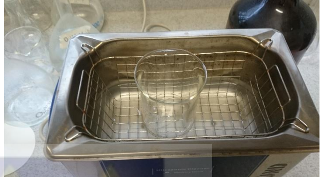
Figure A 2 Cleaning of substrates in an ultrasonic cleaner
