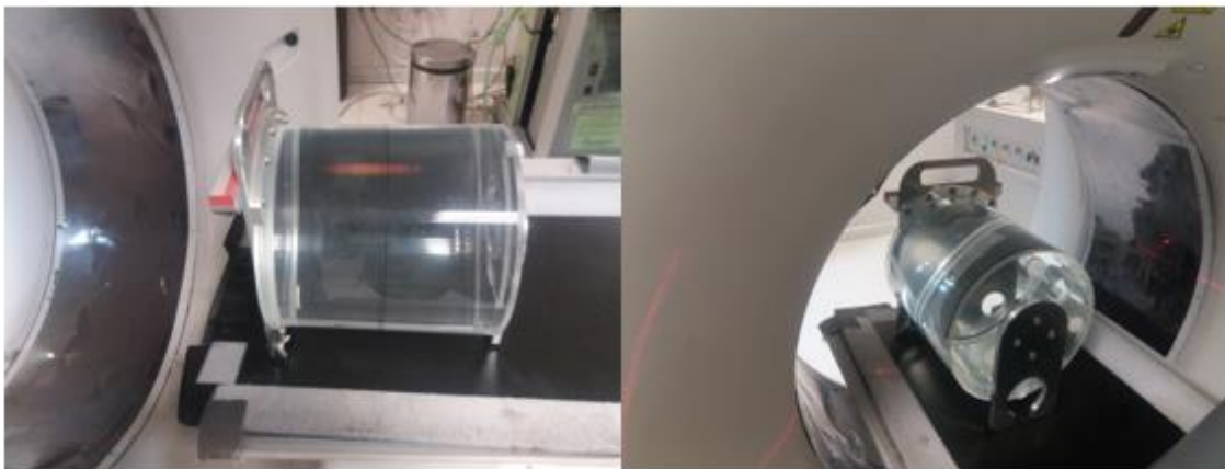
Figure 3.9: Water-filled phantom for CT number, homogeneity and image noise testing.
