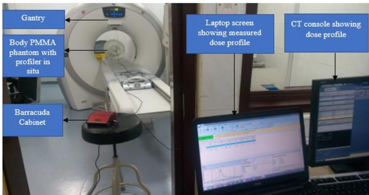
Figure 3.7: Experimental set up for dose delivery accuracy tests. CT: computed tomography
