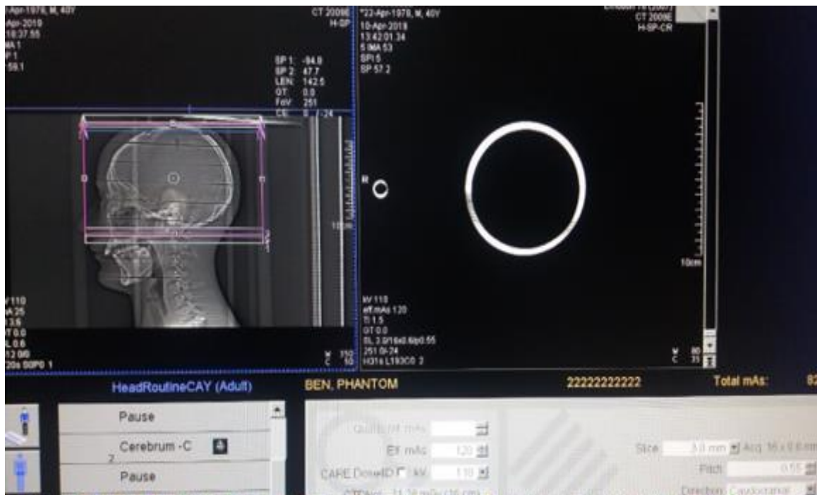
Figure 3.16: Scan coverages used in scanning the Alderson RANDO phantom.
