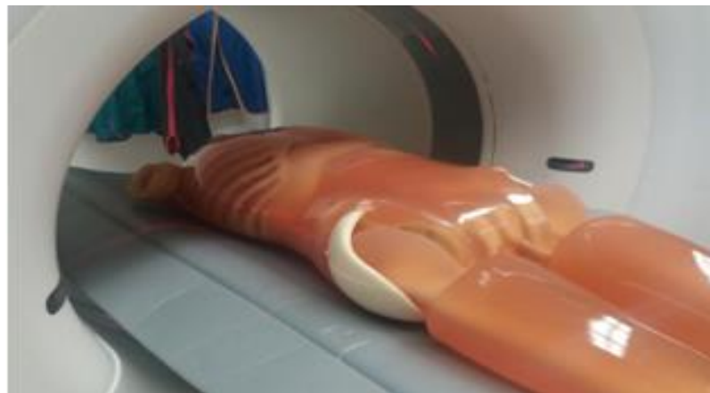
Figure 3.20: Positioning of PBU-60 phantom for AEC studies
