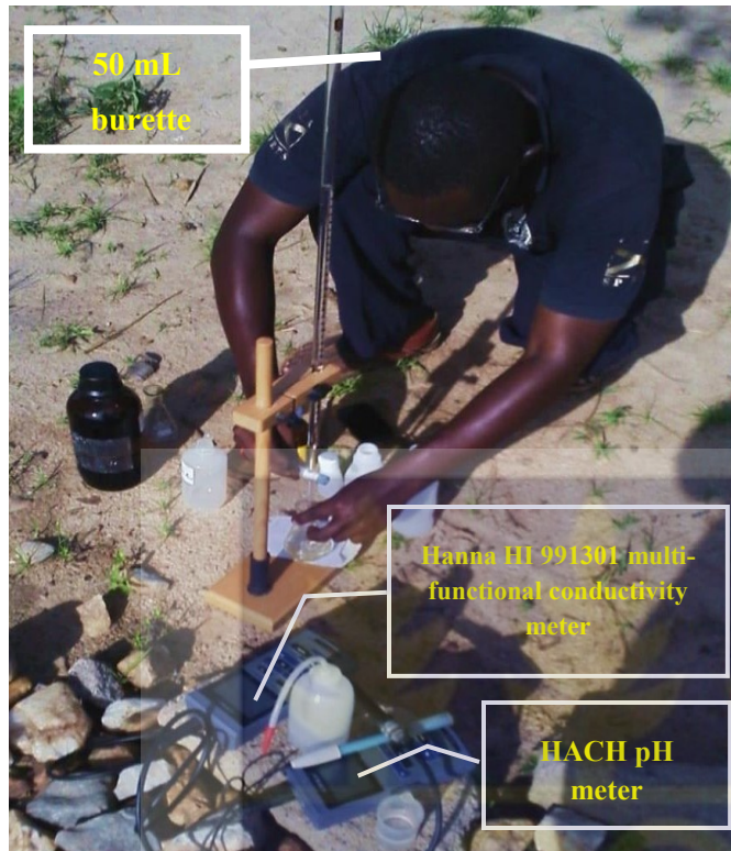
Fig 3.5: On-site Alkalinity determination
