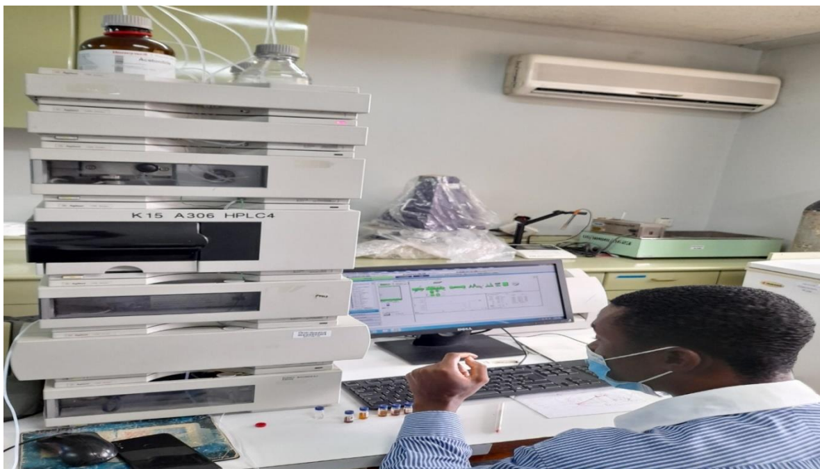
Plate A4: Analysing herbal products for fingerprints using K15 A306 HPLC4 Machine.
