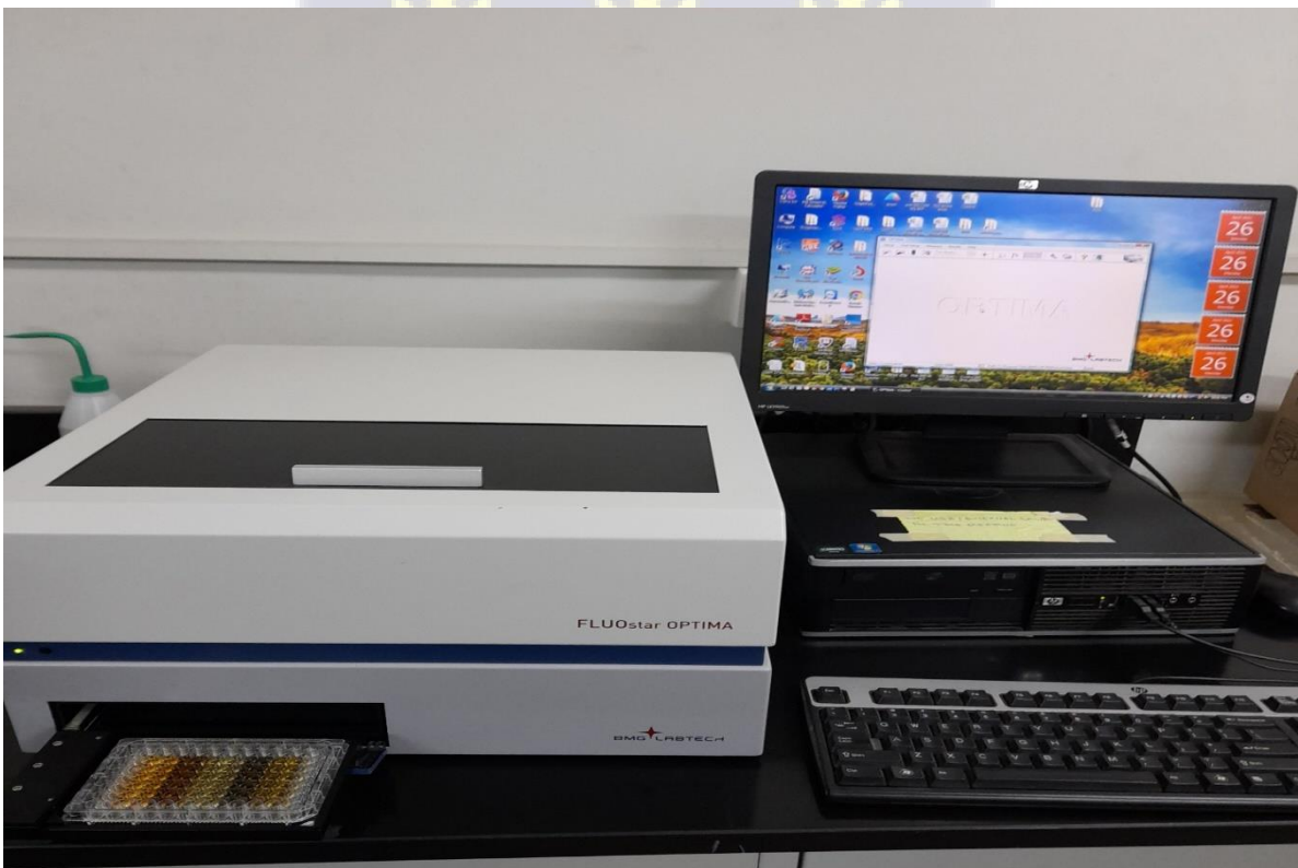
Plate A3: Reading drug plate with Fluostar Optima Plate Reader
