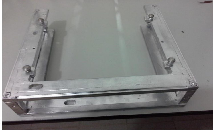
Plate 3.14 Leaf frame designed to hold the leaves locally
