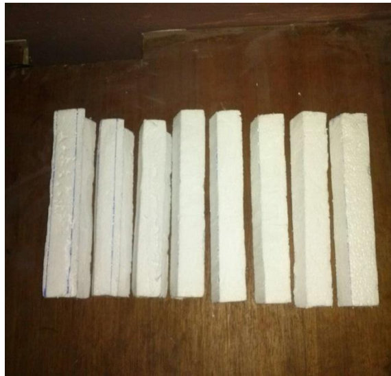
Plate 3.6a. Initial styrofoam designs to mimic the original collimator “leaves”.
