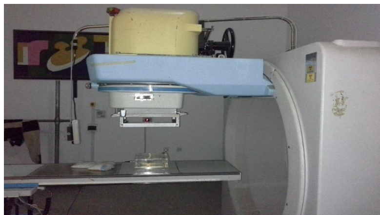
Plate 3.5 Practical setup of the QC measurement with solid water phantom.
