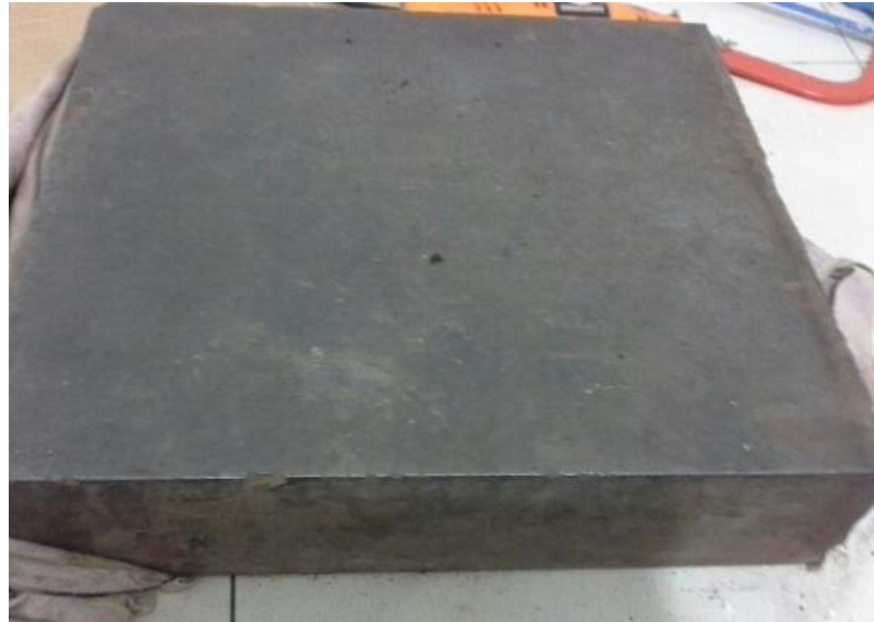
Plate 3.0 High carbon steel alloy used for the fabrication of the MLC
