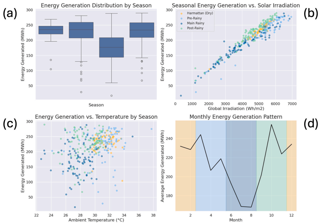
Fig. 10. Seasonal characterization of energy generation: (a) Distribution by season, (b) Relationship with solar irradiation, (c) Temperature dependence by season, and (d) Monthly generation pattern with seasonal transitions.
