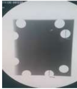
Figure 3.14: Radiograph from the beam collimation check
