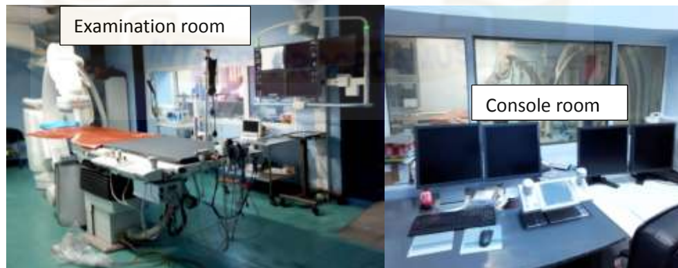
Figure 3.4: Internal view of Cathlab with Siemens biplane fluoroscopy unit.
