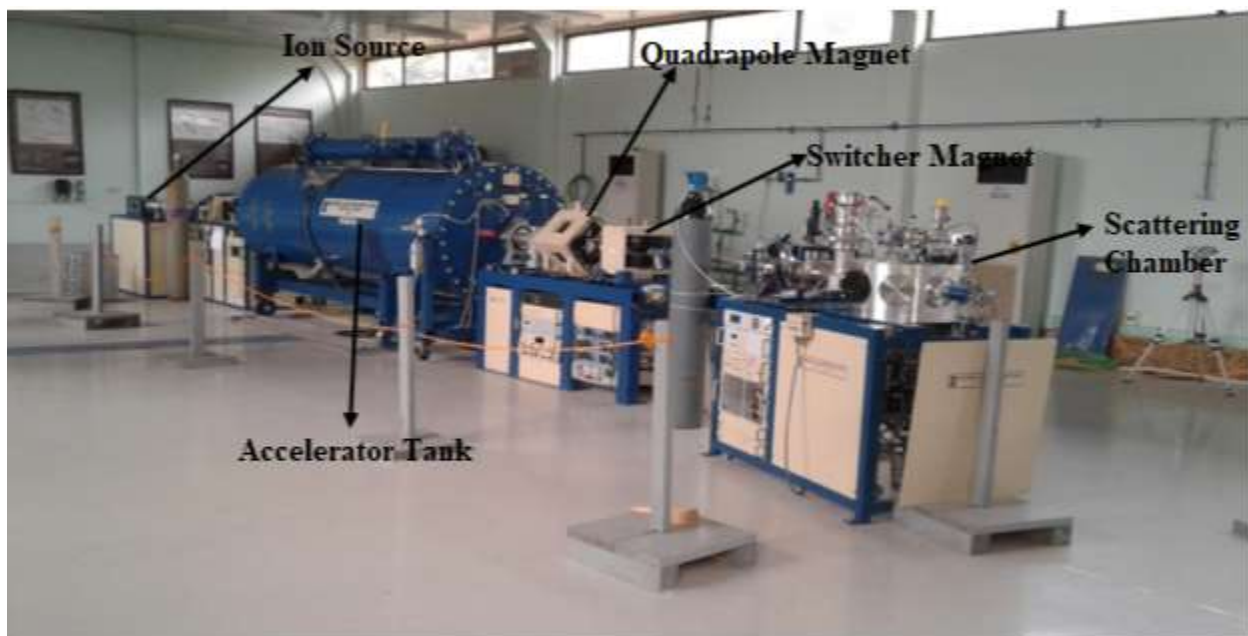
Figure 3. 1: Setup of the 1.7 MV Pelletron accelerator at the Ghana Atomic Energy Commission
