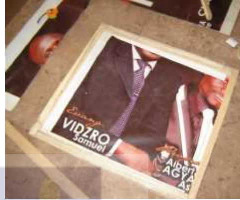
Figure 36. PVCS nailed unto a wooden frame forming single noise insulating panel.
