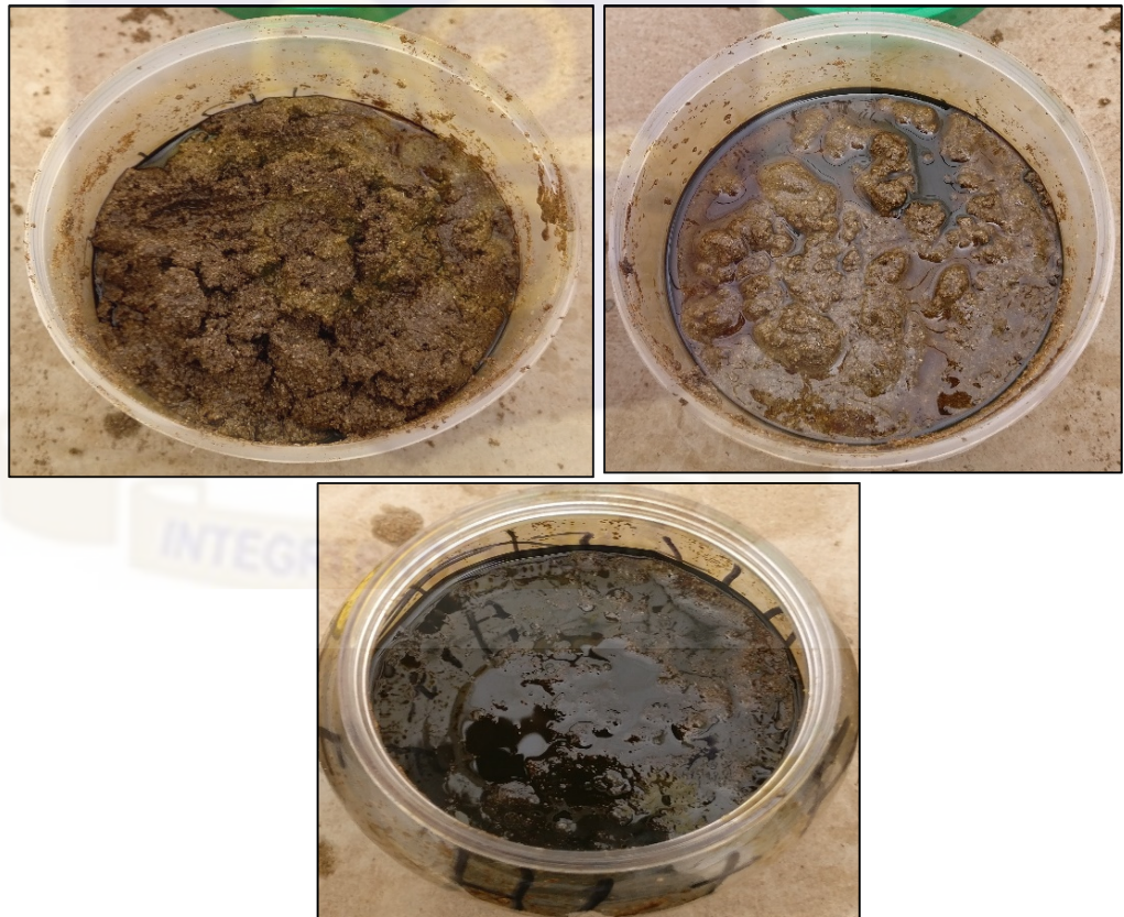
Figure 7.5.7: Nature of hydrocarbon contaminated soil 48 hours after treating with hydrogen peroxide and fertilizer
