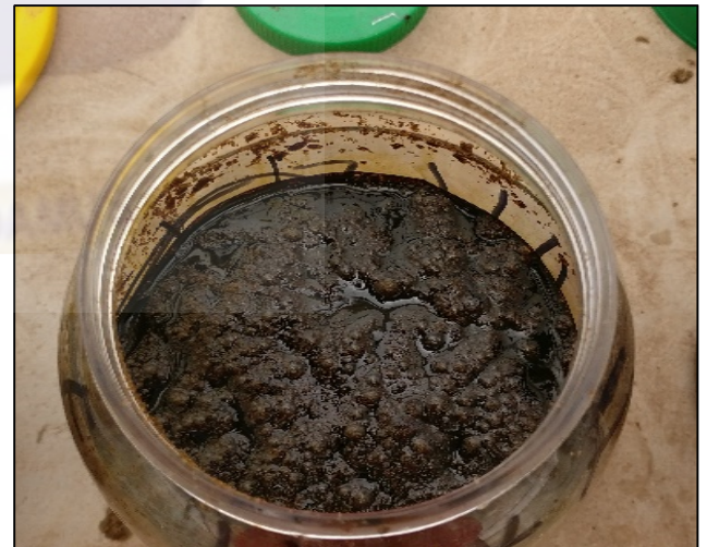
Figure 7.5.2: Hydrocarbon contaminated soil reacting to the addition of hydrogen peroxide
