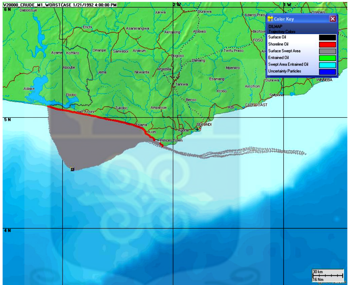
Figure 2.2.1: Trajectory of 168-hour spill of 20,000 Tonnes Crude from Jubilee field
