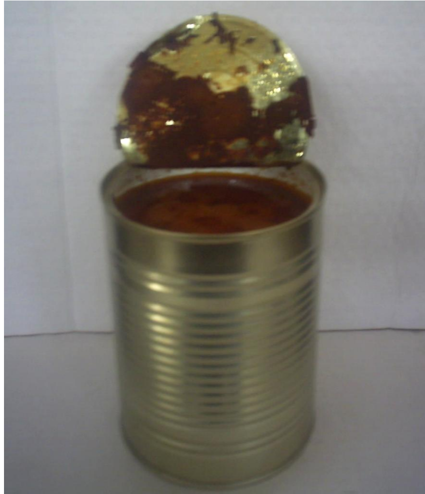
Plate 2: Canned peanut soup base with 3.75% covering oil showing lid darkening effect after retorting at 115°C for 50mins
