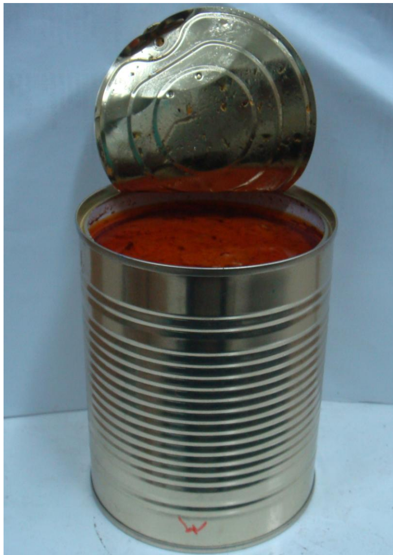
Plate 3: Canned peanut soup base with 3.75% covering oil without lid darkening effect after retorting at 115°C for 40mins
