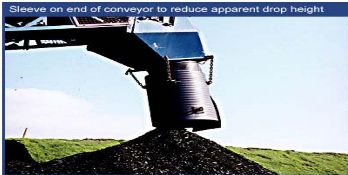
Plate 24: Sleeve on end of conveyor to reduce apparent drop height
