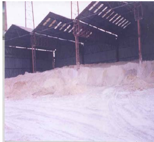
. Plate 26: Stockpiles stored under sheds to reduce fugitive dust emission
