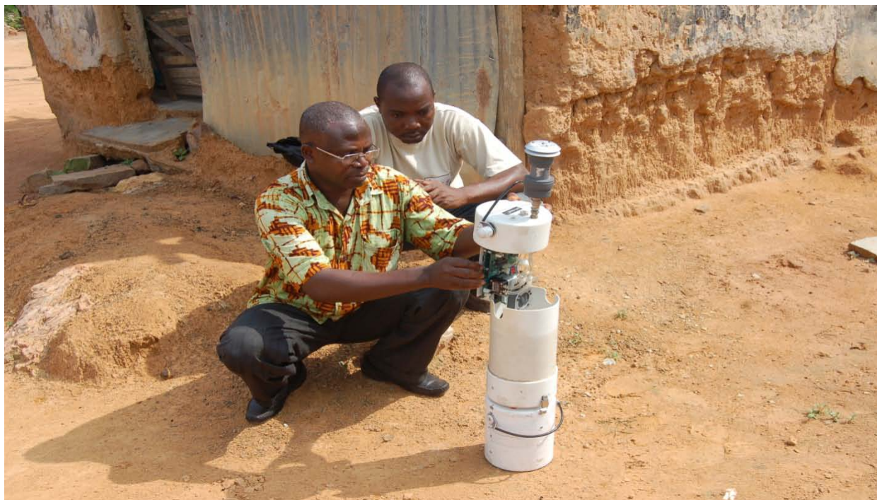
Plate 28: Researcher being assisted by a technician to set the flowmeter and elapsed time totalizer
