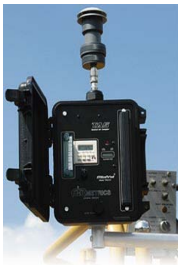
Plate 31: a) Mini- Volume Portable Air Samplers used in sampling PM 10
