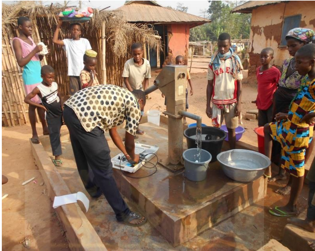
Figure 3.2: Sampling Groundwater using the existing infrastructure
