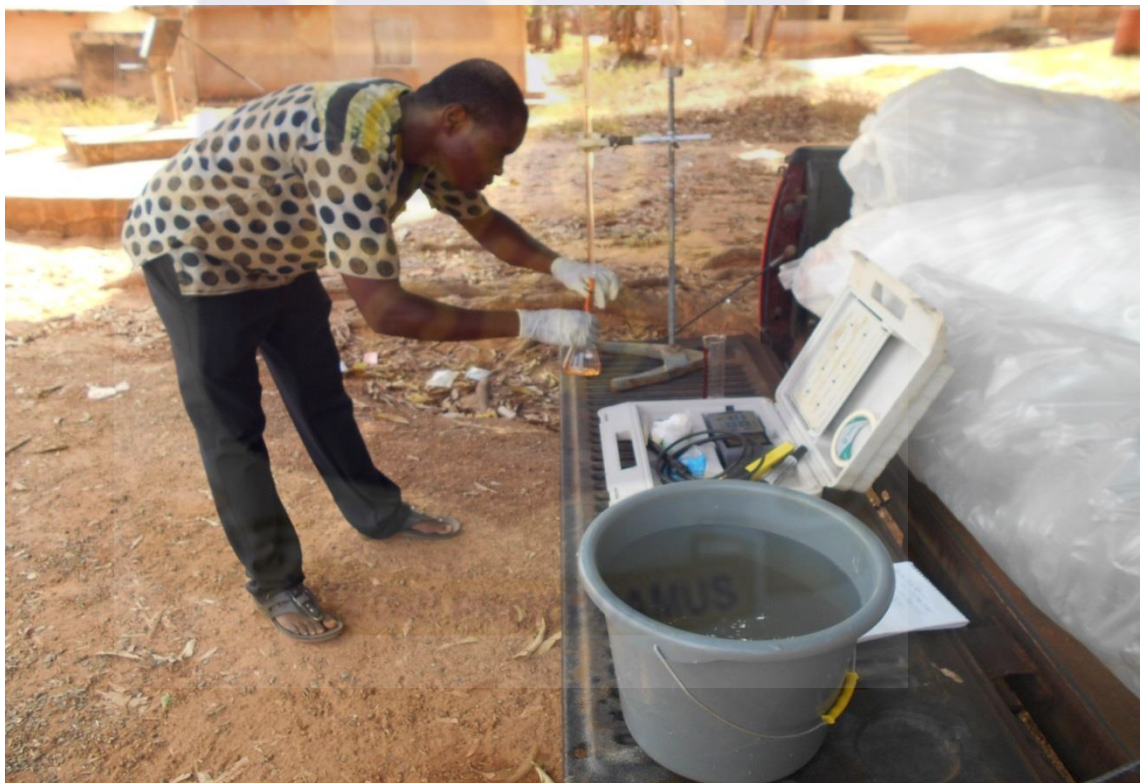
Figure 3.3: Simple titration for determining alkalinity
