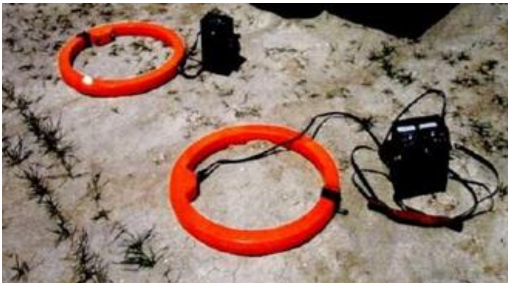
Figure 3 - 1: Image of Geonics EM34-3 system (Xia et al. 2001)
