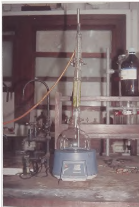
Plate 1a: Photographs showing Soxhlet apparatus used for the acetone and methanol extractions of the test plants ( \times \frac{1}{10} ).
