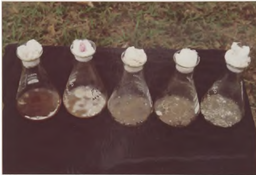
Plate 3: Vegetative growth of P. varioti in Maize meal broth (using Obaatanpa variety) amended with methanol extract of Z. xanthoxyloides and incubated at 28-31°C for 8 days (x 1 / 4 ).
