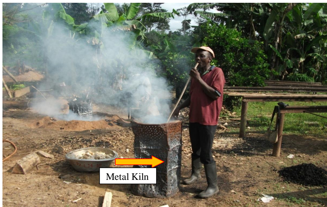
Plate 3.3.1: A photo of a metal kiln and a worker at FOHCREC lighting up fire to heat the kiln before pyrolysis
