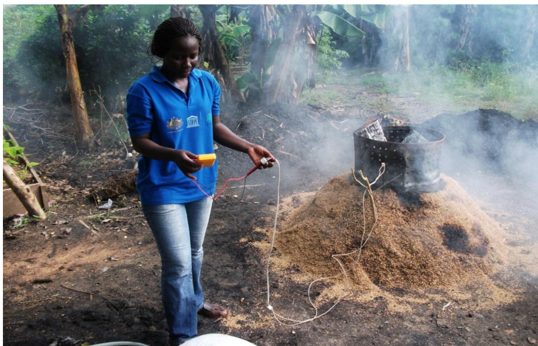
Plate 3.3.3: Measuring temperature using a thermocouple connected to a multimeter.
