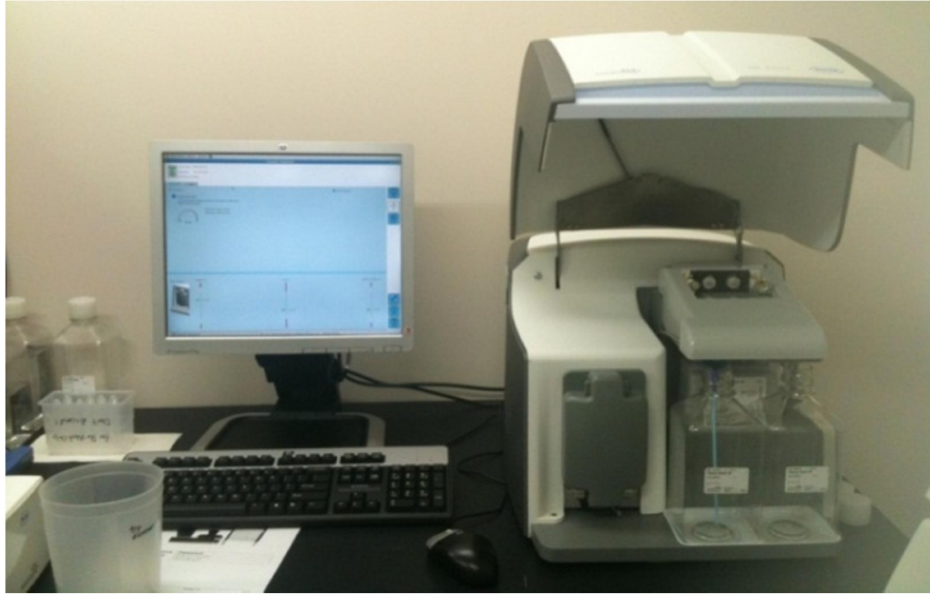
Figure 4: Bench top Next-Generation Sequencer (Roche Genome sequencer junior)
