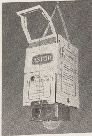
Figure 1 Radiosonde with radiometer attached
