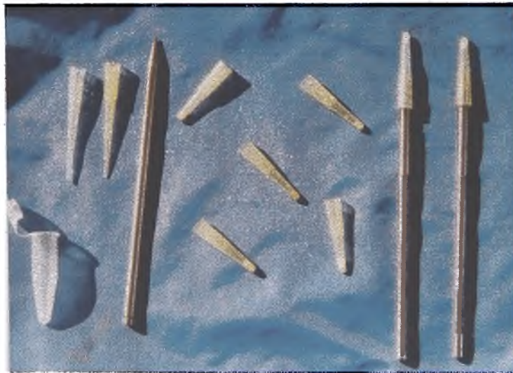
Plate 2: Fabrication of disposable micro-pestle tips left to right: microcentrifuge tube micropipette, micropipette tips, metallic micropestle, moulded micropestle tips, finished tips wedged on to metallic micropestles ready for use.
