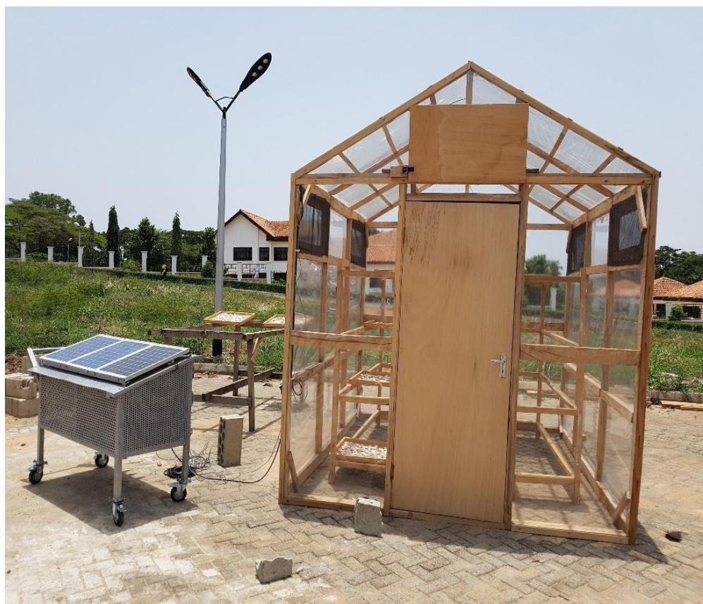
Illustration 19: Complete experimental set-up of the PV-greenhouse solar dryer and the multifunction workstation
