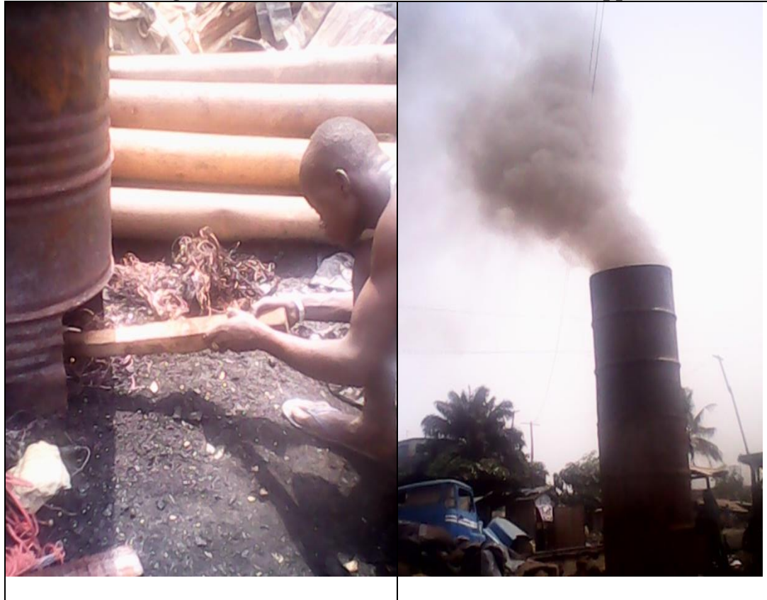
Plate 4.2: Burning of Sheathed Wire at Kumasi to Harvest Copper
