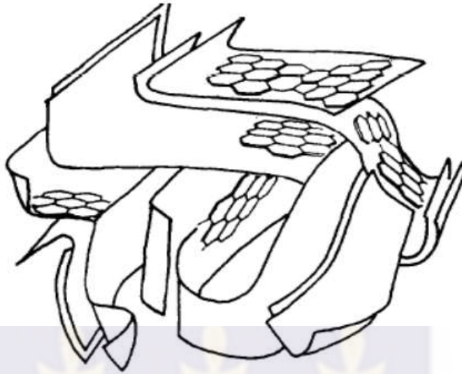
Figure 2.1 Structural representation of activated carbon
