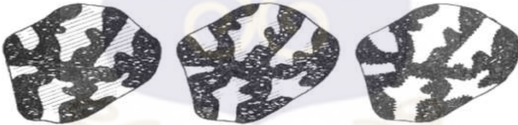
Figure 2.4 Gradual activation process of carbon during thermal treatment
