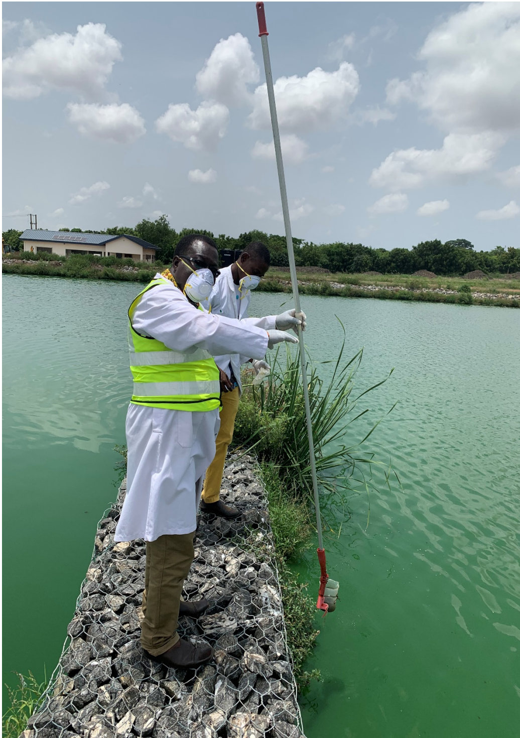
Figure 5: Sampling from the facultative pond
