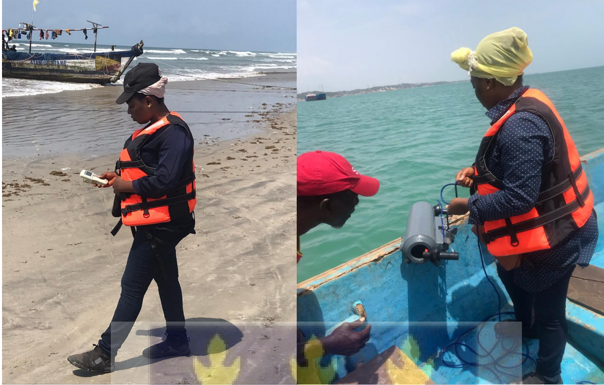
Plate 3.1: Dose rate measurement at 1m above ground surface on the coast. Plate 3.2: Seawater sampling with a Niskin bottle
