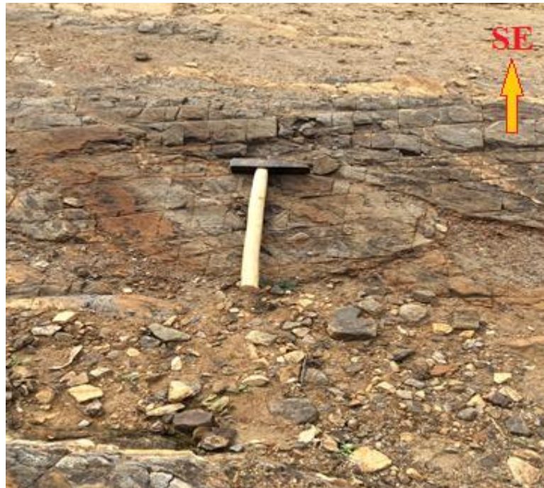
Fig. 4.38. Parallel and perpendicular joint sets intercept orthogonally in the hornblende-bearing gneiss at Torkor. (Picture taken in the direction of dip). Picture taken in the SE direction.
