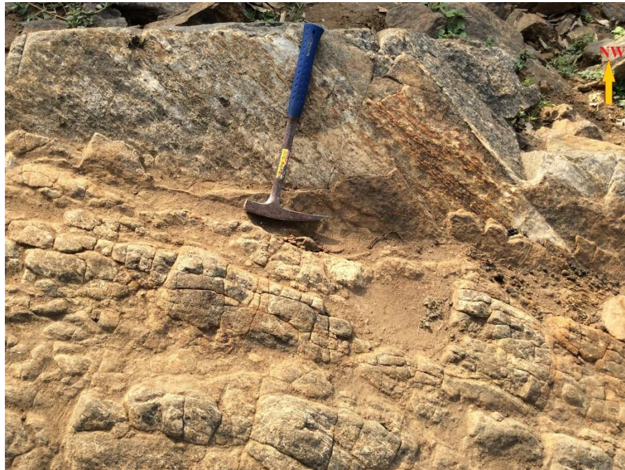
Fig. 4.55. Slickenside with various slickenlines observed closer to the lithologic contact between the ultramafic rock and the hornblende-bearing gneiss at Torkor. This rock also displays parallel set of joints. Picture direction is NW.
