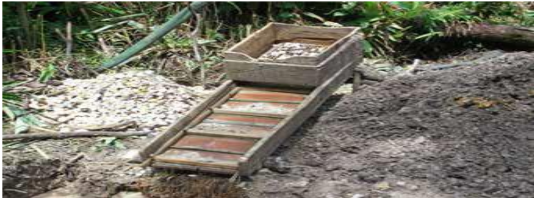
Figure 4: wooden sluice box use by illegal gold miners
