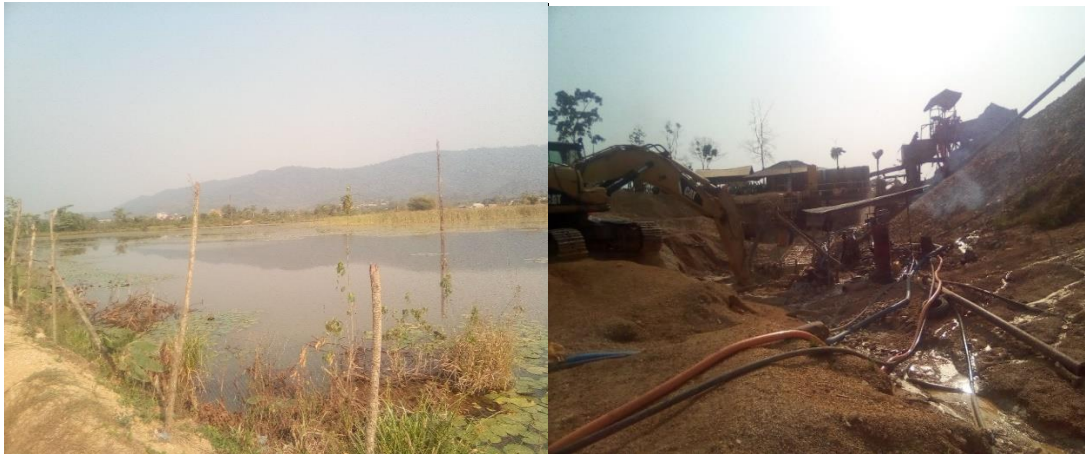
Plate 4.4 Embankment around the tailings dam and spillage from processing pipes at Kwabeng.
