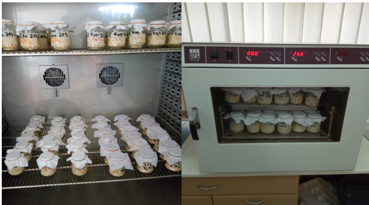
Plate 1: Setup of treated maize samples in incubators at 20°C, 27°C and 31°C
