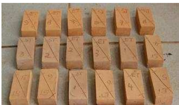
Figure 3. Bauxite Red Mud-Clay briquettes
