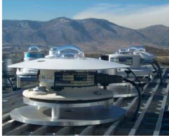
Fig 1.7: Pyranometer for measuring global horizontal radiation. (Adapted from Stoffel and Wilcox, 2004)
