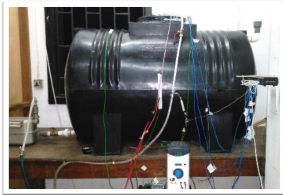
Figure 3-2: The anaerobic digester of the horizontal cylindrical plastic tank with torispherical ends, assembled and operated as a single stage batch system
