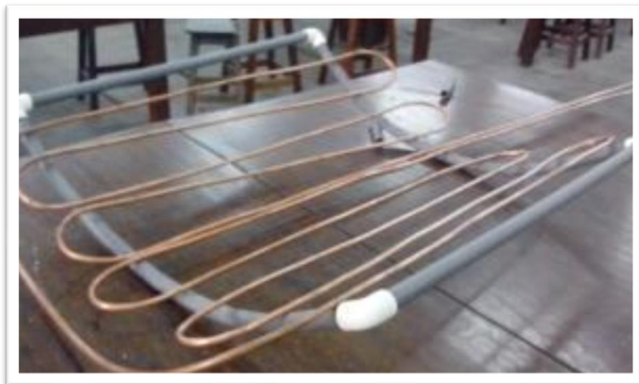
Figure 3-6: Rectangular PVC platform with copper tubing heat exchanger. Distilled water was used as the liquid inside the tube for the heat water circulation
