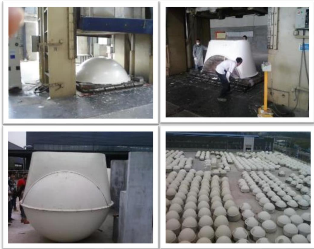
Figure 2-7: Production process of glass fibre reinforced plastic digester with mass production ready for deployment Source: (Hongqi. P. R. C., 2013)
