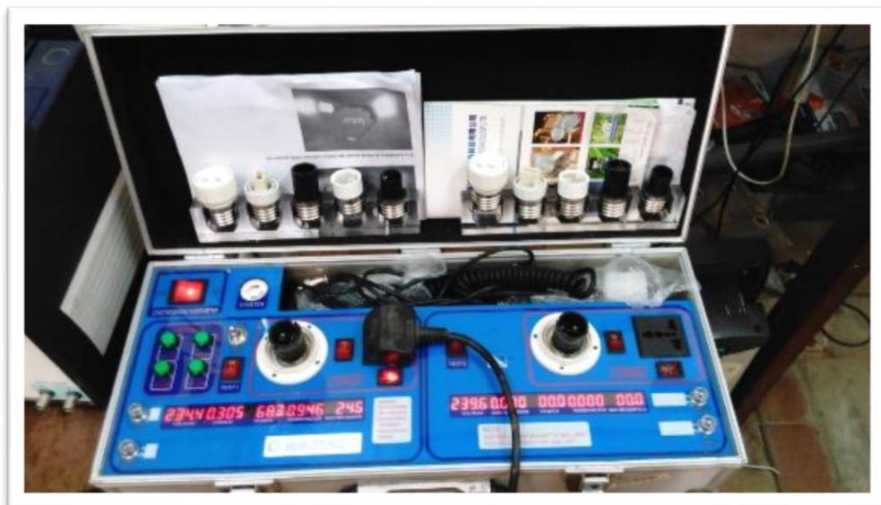
Figure 3-10: A single phase energy monitoring equipment
