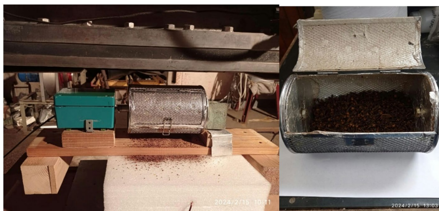
Fig. 1 Irradiation of the cloves with LEEB in rotating cylinder
