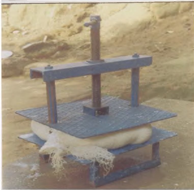
Fig.5 Dewatering of decoloured fermented cassava meal in Akyeke processing
