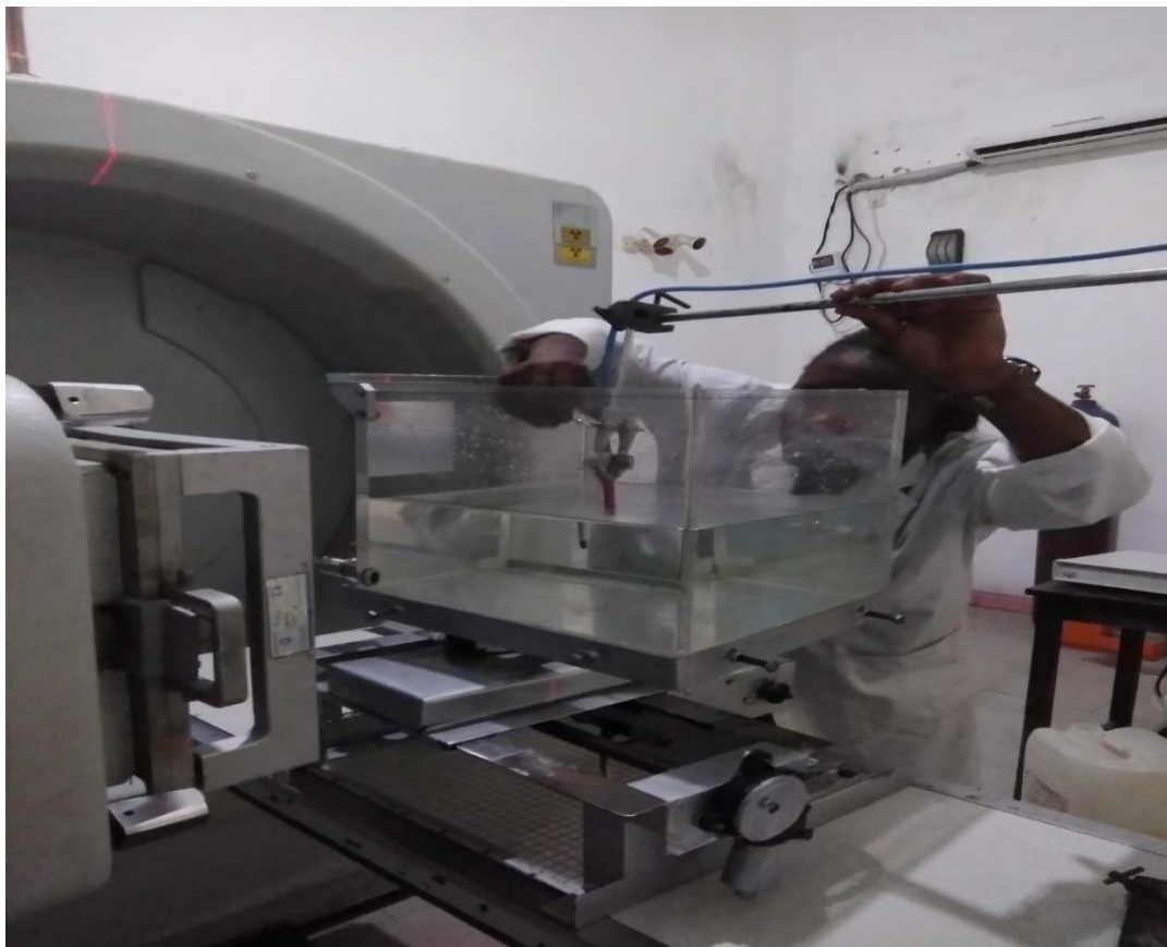
Figure 3. 14- Setup for beam profile measurement
