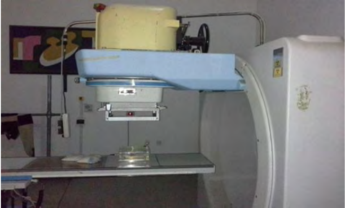
Figure 3. 11 - Practical setup of the QC measurement with solid water phantom
