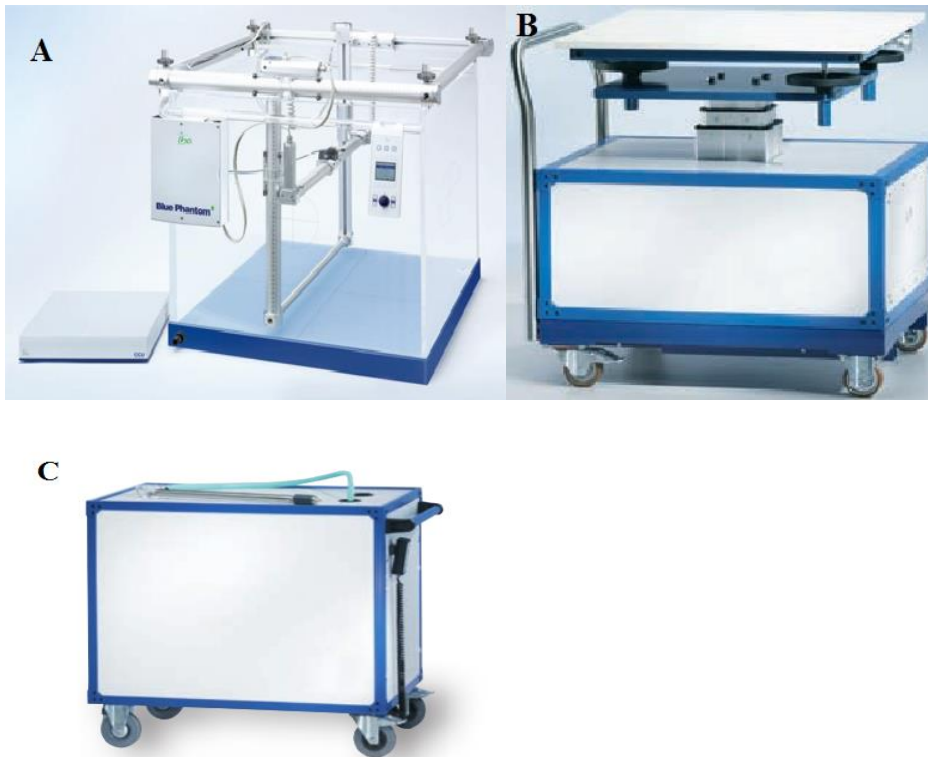
Figure 3.5. Blue Phantom 2 motorized water phantom components; A. water tank, showing leveling knobs for detector holder, common control unit, hand control unit and detector holder mechanism; B. water tank carriage; and C. water reservoir, showing nozzle for filling the water tank on top and an independent hand control to fill and drain the tank at the side.
