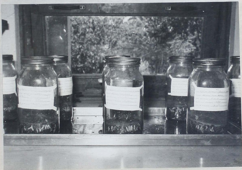
Fig. 8: Experimental glass jars with broken cocoa beans, standing on aluminium tray, flooded with machine oil.
