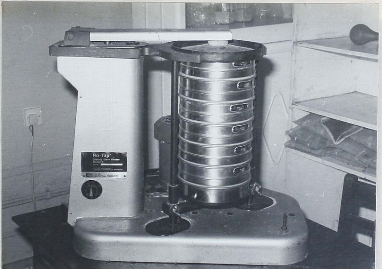
Fig. 5: Ro-tap testing sieve shaker (Model B), used for determining particle size ranges for food medium.
