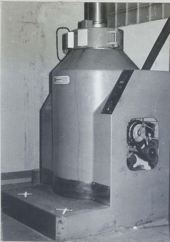
Fig. 12: Gamma cell 220 (Cobalt- 60 irradiator source) at the Ghana Atomic Energy Commission, Kwabenya, used for the radiosensitivity experiments with C. cephalonica .
