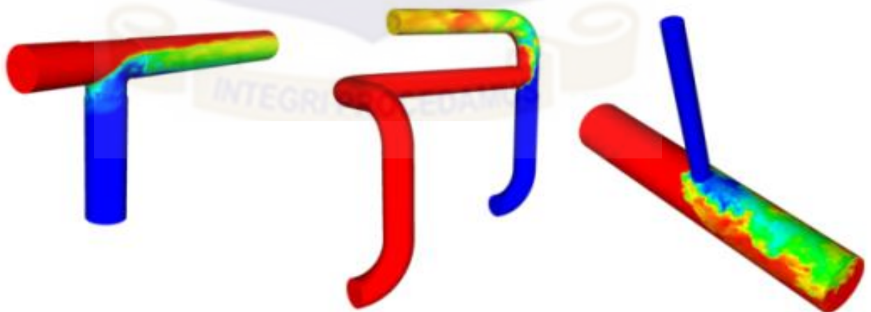
Figure 1.3: Typical T-Junctions that exist in Nuclear Power Plants.
