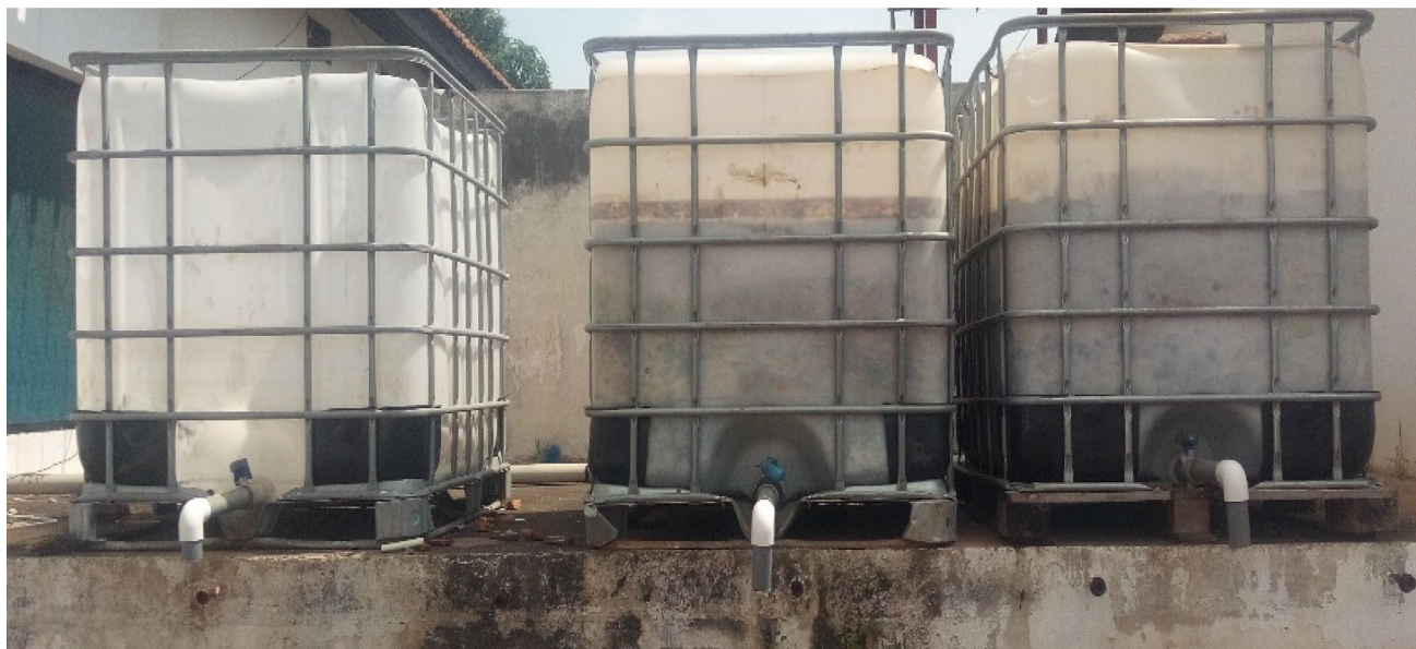
Fig. 6 The wastewater filtration setup at the Agricultural Engineering Workshop
