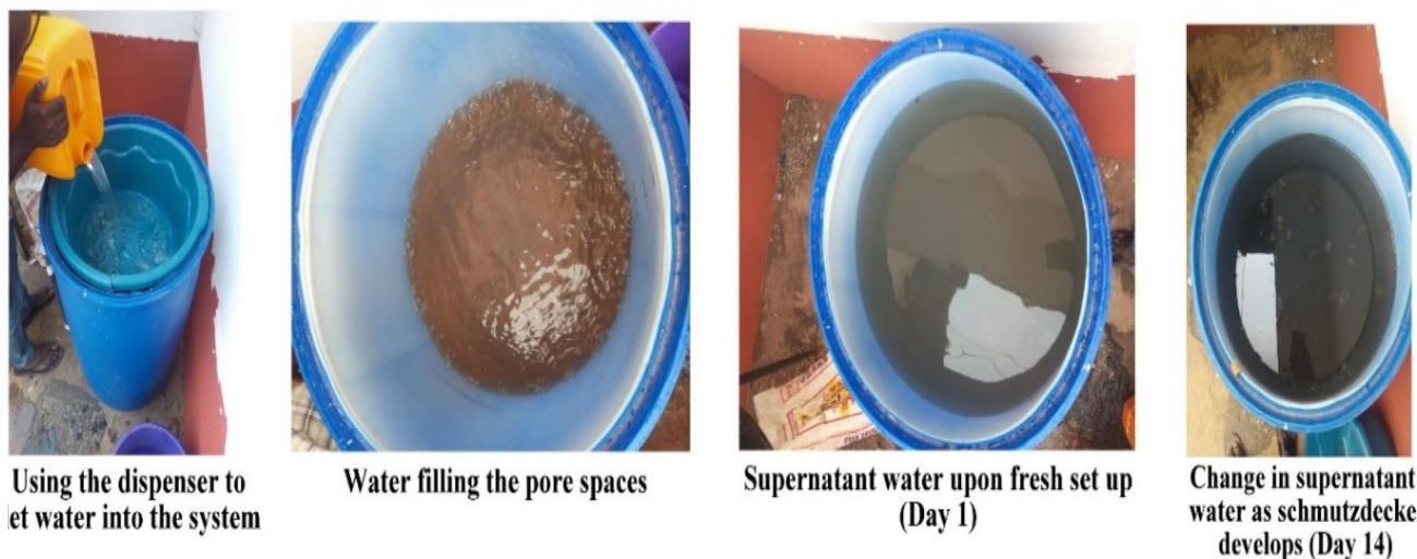
Fig. 4 SSF wastewater filtration process
