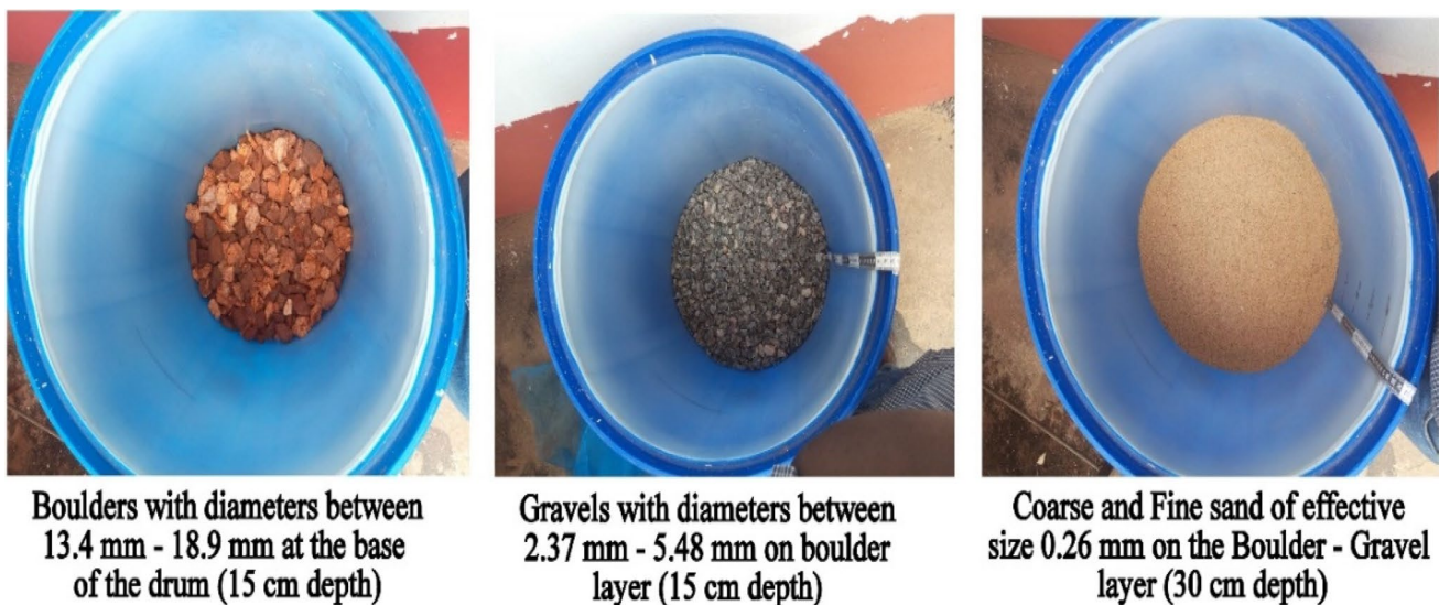
Fig. 3 Arrangement of boulders, gravel and sand in the filter
