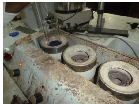
FIG. 3.10d: Pre-heating of analyte for titration
