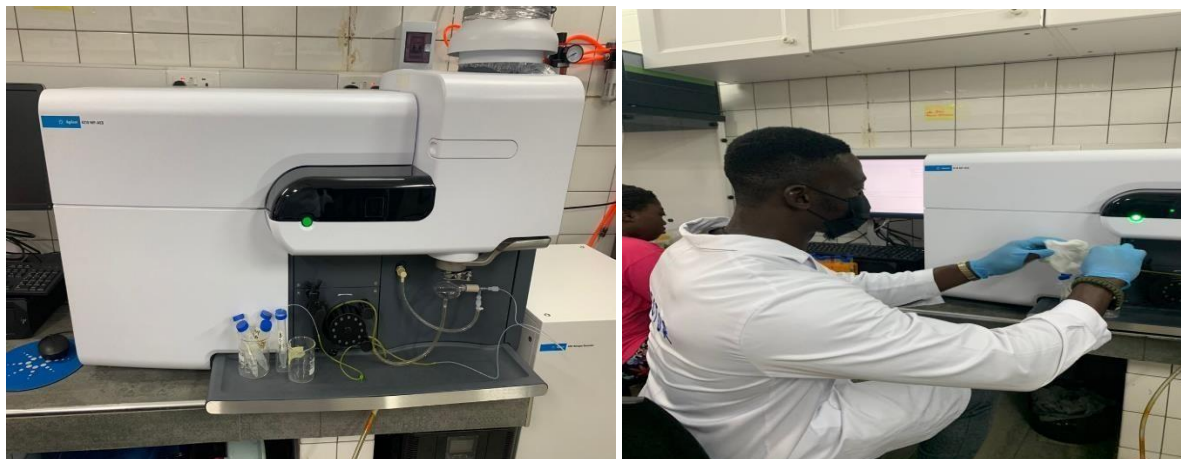
Figure 7. Summary of using the Agilent 4210 MP-AES to analyse for Mg and Ca ions in samples.
