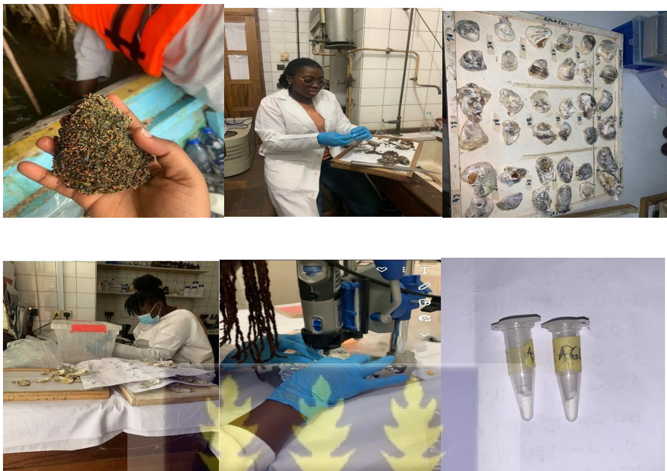
Figure 6: Shucking, cleaning, drying, sectioning, and drilling of oyster shells for laboratory analysis.
