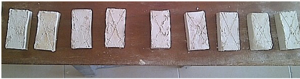
Fig. 9. Green bodies during drying at room temperature.
