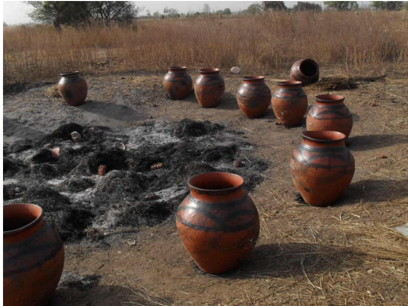
Figure 38: Photo showing fired vessels and post fired treatment with plant solution
