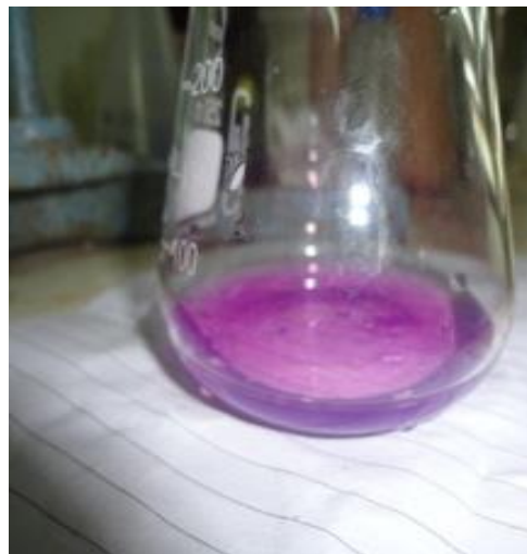
Fig 3.4b: Purple colour developed at the end of titration
