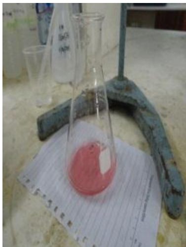
Fig. 3.4a: Mixture of NaOH, murexide indicator and aliquot of water sample
