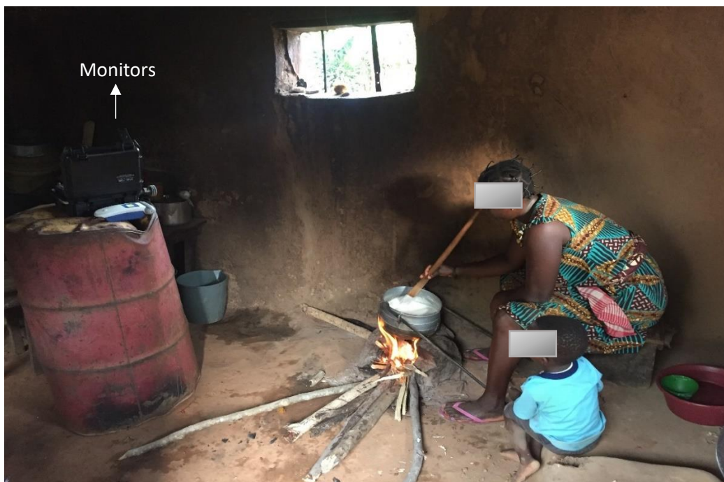
Plate 7: Assessment of Emissions Using EPAM 7500 and Aeroqual S500 Gas Monitor During the Controlled Cooking Test.
