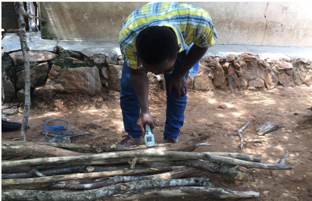
Plate 5: Assessment of Fuelwood Moisture Using Wood Moisture Meter
