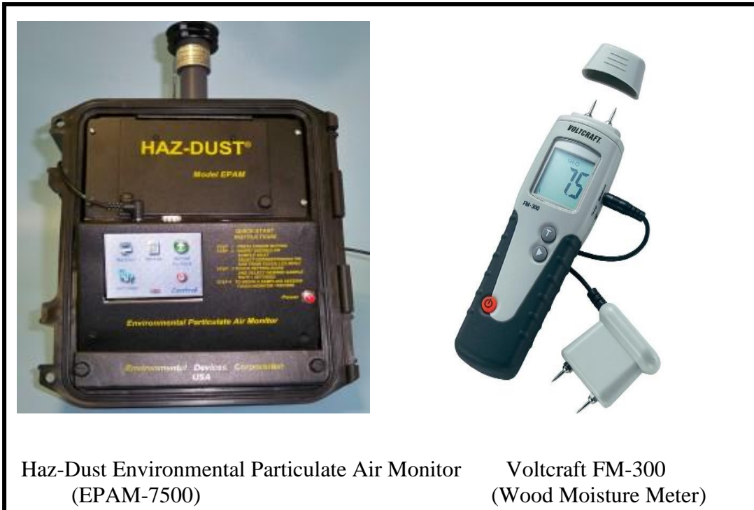
Plate 4: Haz-Dust Environmental Particulate Air Monitor (EPAM-7500) and Voltcraft FM-300 (Wood Moisture Meter)
