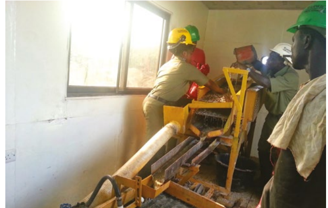
A locally manufactured mineral table using the principle of gravity for the separation of gold in the ore A simple process that can replace the mercury commonly used in the galamsey gold operators
