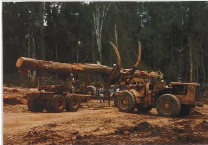
Figure 12. Front-end loader loading extracted boles onto a haul truck.
