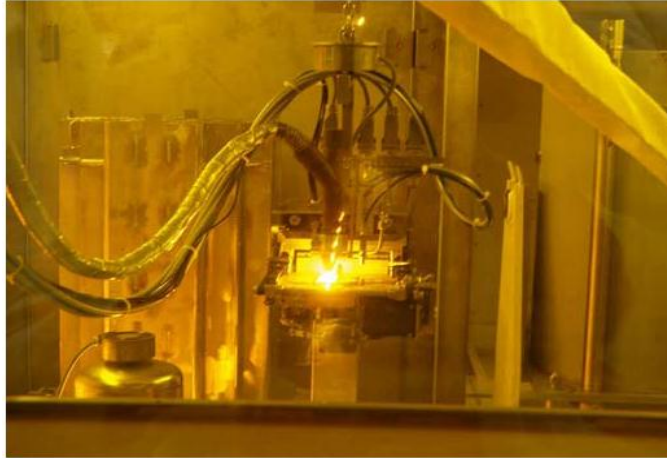
Figure 2.5: Welding of canister with EK-10 FA inside the hot cell
