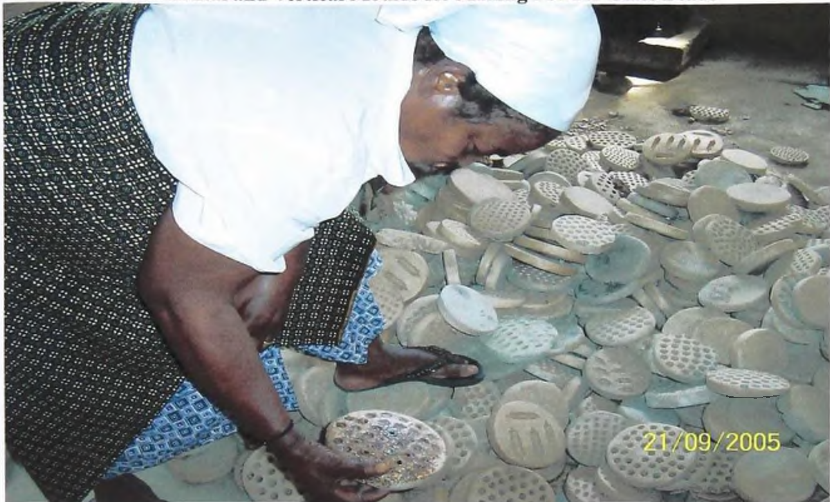
Plate 3.14 Horizontal and Vertical Moulds for Making Powder Glass Beads
